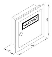
Open central control and remove the housing top section (door) from the housing bottom section. Fasten the housing bottom section in the wall cut-out (cut-out dimension 335 x 350 x 95) and refit the housing top section.
