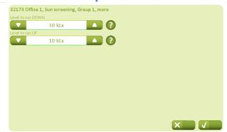
The light levels for deployment and withdrawal of sun screening product respectively must be configured. In order to avoid cyclical variation of the sun screen product, it is recommended that the values should not be too close together.
