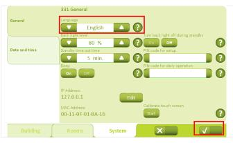
The "General" tab can be used to configure: language, background illumination, the time after which the background illumination will go into sleep mode, the beep sound when the keys are used and the PIN code for super-user and end user respectively.
