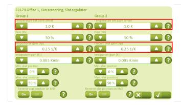
The tilting of the slats must be configured under the tab "Sun screening" – "More". The tilting is based on temperature measurements in the room.
