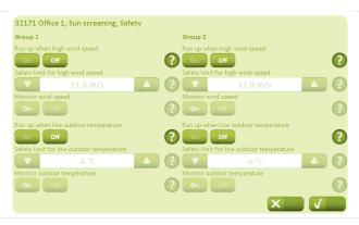
For the protection of the sun screening product, it is recommended that the sun screening product is withdrawn in the event of either high winds or low temperature.
