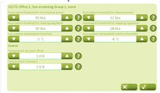
Temperature and illumination set-points must be defined based on when they contribute positively or negatively to the building's room temperature.
