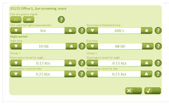
The "Night period" must be defined on the tab "Sun screening" – "More", either with fixed times or by defining lighting levels. If "Screen due to night" is activated, the sun screen product will be deployed during the defined night period.
