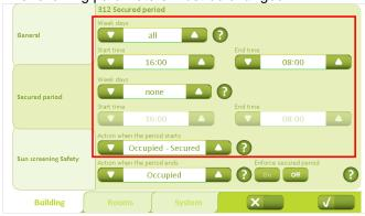
The time periods for the different operating modes must be configured here. For example, two different times can be defined: one for working days and one for weekends.
