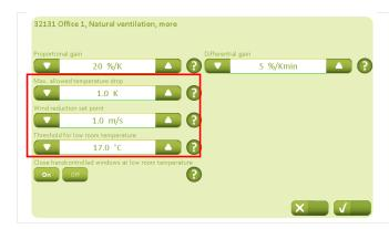
The maximum temperature drop compared to the temperature set-point defines when the windows must be closed. This is particularly important for ventilation with fixed times.
