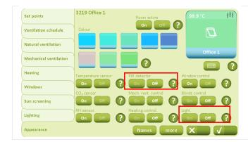
On the "Appearance" tab, the "Lighting control" and "PIR sensor" must be set to "On" in all rooms in where lighting control is required.
