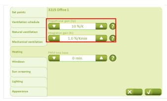
It is recommended <u>not</u> to set the proportional gain too high on the "Heating" tab, e.g. 50%/K, as this can result in instability/cyclic variation.
