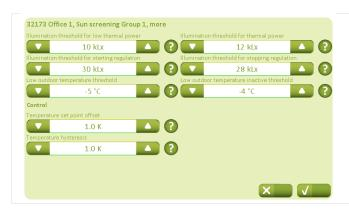
The temperature and lighting set-points must be defined on the tab "Sun screening" – "More" based on when light levels and outdoor temperature contribute positively or negatively to the building's room temperature.
