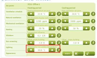
The "Set-points" tab is used to configure the "Threshold for low outdoor temperature", which defines the temperature at which the system shifts between summer and winter operation.
