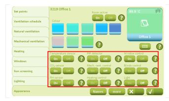
Since only one temperature-dependent ventilation is required, "CO<sub>2</sub> sensor", "RH sensor", "PIR sensor", "ventilation control" and "heating control" must be set to "Off".
