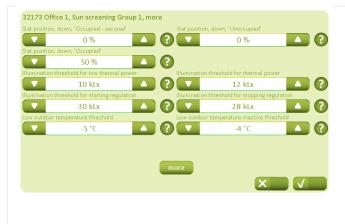
The slat position (horizontal or vertical) when the slats are deployed in the different operating modes must be defined under the tab "Sun screening" – "More".
