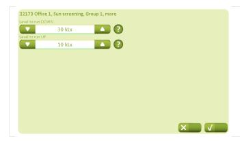
Lighting values for when the sun screen product can be deployed / withdrawn must be defined on the tab "Sun screen" – "More".
