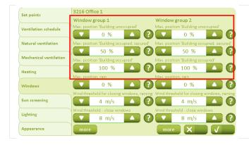
The window's maximum opening for the individual room and operating mode is configured under the "Windows" tab.
