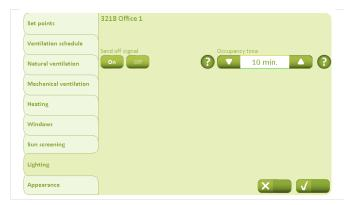
On the "Lighting control" tab, the "Send off signal" must be set to "On" in all rooms if lighting control is required.
