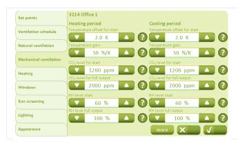
The "Mechanical ventilation" tab is used to define the mechanical ventilation set-points for the heating and cooling periods respectively. The set-point for "Temperature offset for start" is based on the ventilation temperature set-point, which is defined under "Set-points". See section 5.1.1.
