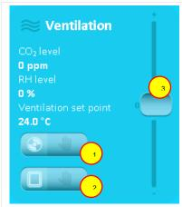
1 Mechanical ventilation - manual operation
