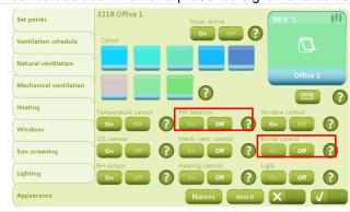
In addition to the sensors/functions that are already activated in connection with ventilation and heating control, the "Blinds control" must be set to "On".
