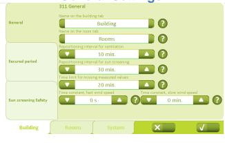
Under the "Building" – "General" tab, the building tab can be renamed and the time interval for the natural ventilation can be defined.
