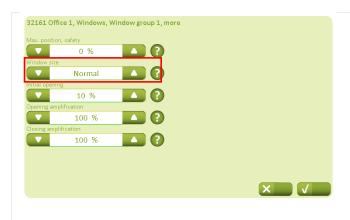
For Natural Ventilation to function, it is necessary to have a sufficient number of motorised windows in the building. For NV Comfort™ to be configured to switch optimally between ventilation and Comfort™ it is important that the windows used in a zone are correctly configured in relation to each other.
