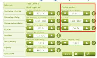
The set-points for summer operation are indicated under the "Set-points" tab and the "Cooling period" heading.
