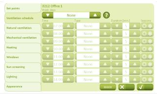
The time/length of the airing/ventilation and the time at which the ventilation should occur are configured on the "Ventilation times" tab.
