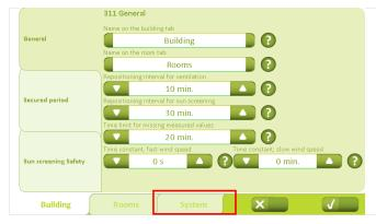
Use the "System" tab to choose between several different tabs for setting parameters.
