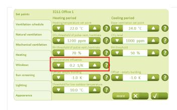
The "Temperature influence" value is used to determine whether pulse ventilation should also be used in winter when the temperature set-point, the relative humidity set-point or the CO<sub>2</sub> set-point is exceeded.
