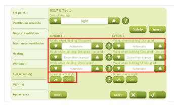
The "Sun screening" tab is used to define how the sun screen products are to be controlled in the different operating forms.
