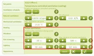
The "Natural Ventilation" tab is used to configure whether requirement-controlled pulse ventilation should be used.
