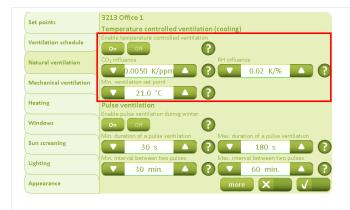
Enable whether the ventilation is to be temperature based or not. The effect of the  $CO_2$  content and the relative humidity on the desired set-point to be calculated are configured under the "Natural Ventilation" tab, if the previously set limits are exceeded, the system reduces the temperature set-point in accordance with the settings.
