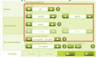
The time periods for the different operating modes must be configured here. For example, two different times can be configured: one for working days and one for weekends.
