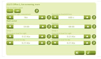
If a PIR sensor is used, "Use occupancy signal" must be set to "On".
