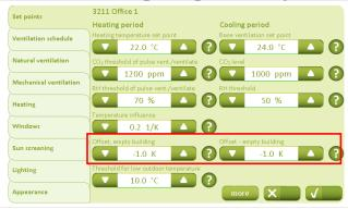
NV Comfort™ allows the lowering of the temperature set-point either to perform night cooling in summer or heat conservation in winter. The fields for temperature displacement "empty building" under the "Set-points" tab can be used for this purpose.
