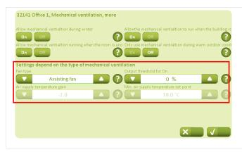
On the "Mechanical ventilation" "More" tab it is defined whether a ZoneVent™ or an assisting fan is used. It is not possible to use both an assisting fan and ZoneVent™!
