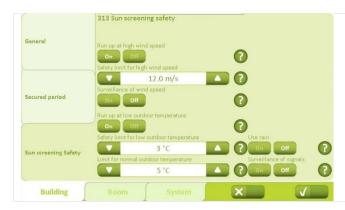
The "Sun Screening Safety" tab under "Building" is used to configure the safety set-points generally for the building.
