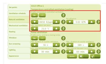
Enable whether the ventilation is to be temperature based or not. The effect of the CO<sub>2</sub> content and the relative humidity on the desired set-point to be calculated are configured under the "Natural Ventilation" tab, if the previously set limits are exceeded, the system reduces the temperature set-point in accordance with the settings.
