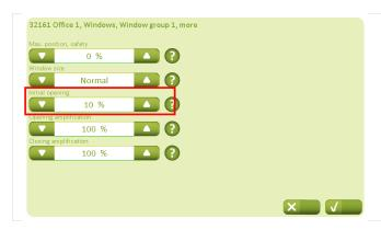
The value "Initial opening" defines the window's opening, which must be performed at the first airing after the windows have been completely closed, e.g. to release the window's gaskets from the frame.
