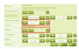
The "Minimal ventilation set-point" can be configured as required. Be aware that it must be at least 2K higher than the "Set-point for low room temperature" (screen image under "More"), as this could otherwise cause cyclical variation.
