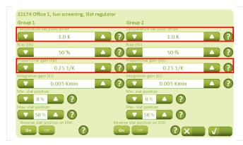
The tilting of the slats must be configured under the tab "Sun screening" – "More". The tilting is based on temperature measurements in the room.
