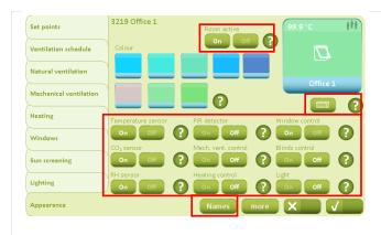
Press "On" in the room menu under the "Appearance" tab. The room is thereby activated.
