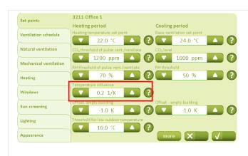
The "Temperature influence" value is used to determine whether pulse ventilation should also be used in winter when the temperature set-point, the relative humidity set-point or the  $CO_2$  set-point is exceeded.
