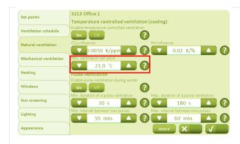
Under the "Natural Ventilation" tab, "Min. ventilation temperature set-point" defines the minimum ventilation set-point the system may use.
