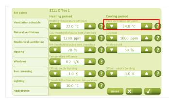
In the "Cooling period", the "Basic ventilation set-point" can be defined for the each room as required.
