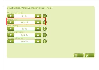
For Natural Ventilation to function, it is necessary to have a sufficient number of motorised windows in the building. For NV Comfort™ to be configured to switch optimally between ventilation and Comfort™ it is important that the windows used in a zone are correctly configured in relation to each other.
