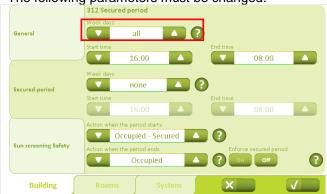
"Week days" must be changed from "all" to "none" under operating modes. In other words, there are no times where there is no ventilation if this is necessary according to the temperature.
