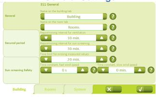
Under the "Building" – "General" tab, the building tab can be renamed and the time interval for the natural ventilation can be defined.
