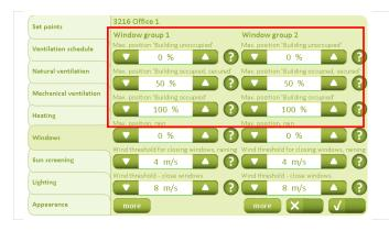
The window's maximum opening for the individual room and operating mode is configured under the "Windows" tab.
