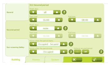
Under the "Building" – "Secured period" tab, secured periods can be defined using days and times.
