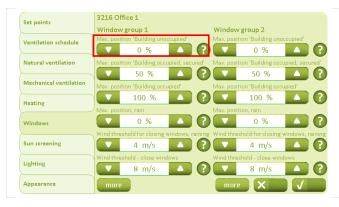
The window parameters for the different rooms can be adapted here.
