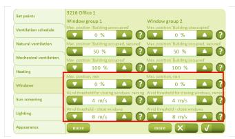
The maximum opening of the window in the event of rain is configured on the "Windows" tab.
