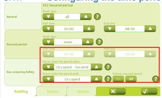
The time period for the automatic change between operating modes is configured under the "Building" – "Secured period" tab.
