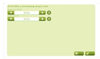
Lighting values for when the sun screen product can be deployed / withdrawn must be defined on the tab "Sun screen" – "More".
