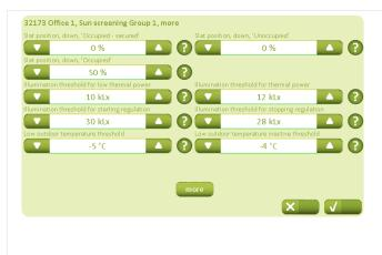
The slat position (horizontal or vertical) when the slats are deployed in the different operating modes must be defined under the tab "Sun screening" – "More".
