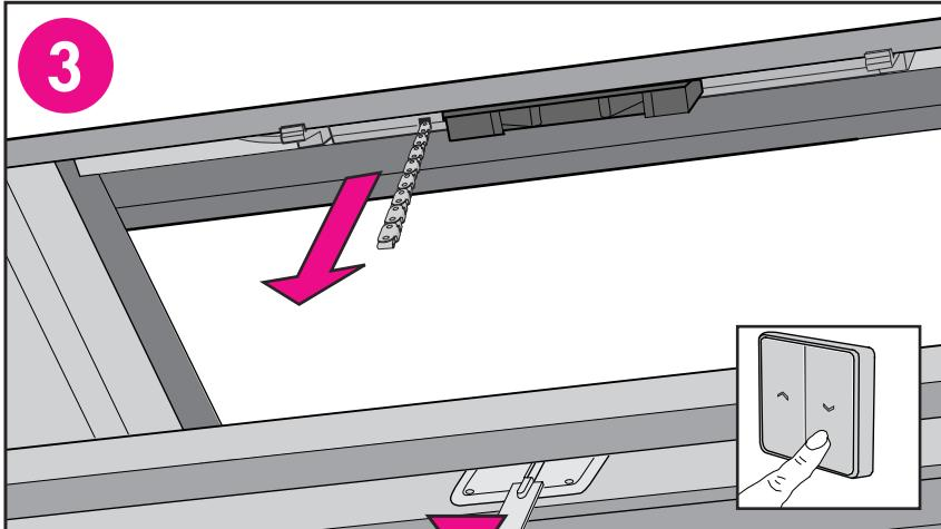
**English:** Close ventilation flap. Locate end of chain in sash bracket U profile and insert retaining clip. Open ventilation flap; the window is now ready for use.
