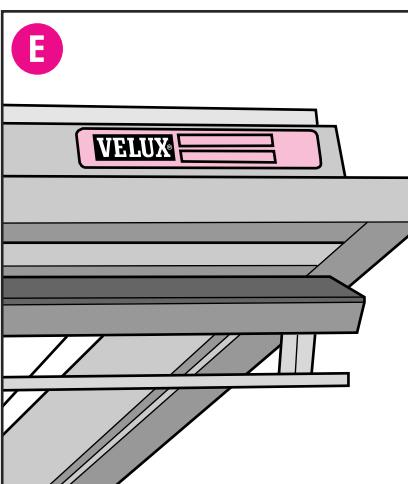
**English:** The window must be brought back to its original appearance (before installation of the first motor). The following components will be required: headlock(s) (**A**), striking plate(s) (**B**), friction springs (**C**) and ventilation flap (**D**). These components are available from WindowMaster. When ordering please state window type and size (see data plate on window top sash (**E**)).
