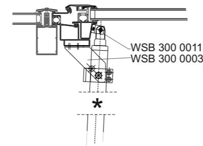
**UK:** Notice the length and the working area of the spindle actuator
