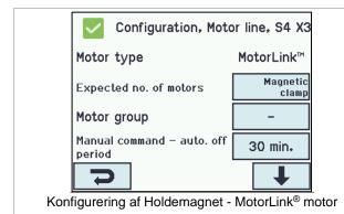
Each motor line (MotorLink®) which is configured as a magnetic clamp must be associated with a motor group.
