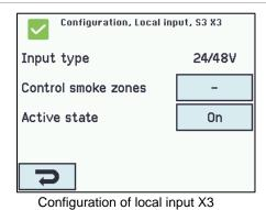
Input X3 on WSA 5IO (24V/48V) (primary used in France) If there is connection in X3 on the module WSA 5IO, it shall be configured in:
