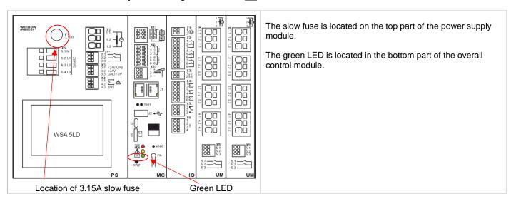
Both fuses are common fuses and can be purchased in by distributors of electronics.
