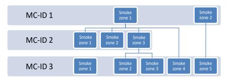
Break glass units and input assigned to a slave-smoke zone are automatically sent to the master smoke zone. They are in the evaluation of smoke on equal level as the local input on the master. The master sends the smoke commands to slaves, which only receive input from the master. To get the fastest response, it is recommended that break glass units are assigned to the section in which the master belongs.
