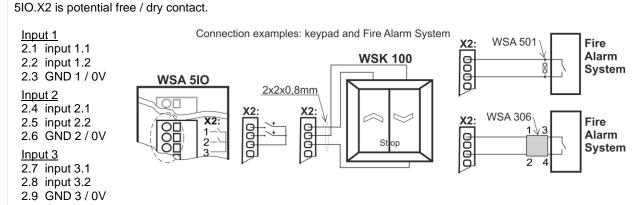
Fire Alarm System shown with cable monitoring type 1 and type 2:
