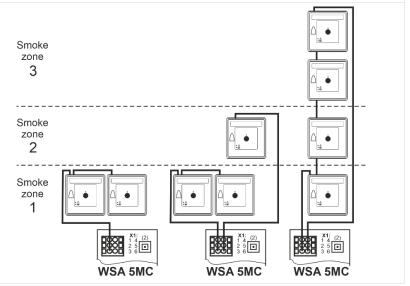
Smoke detectors and keypads are connected on the break glass unit type WSK 501/502.
