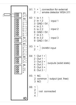
**X1** For connection of smoke detector type WSA 311.
