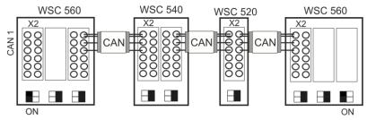
First and last bus-termination must be ON.
