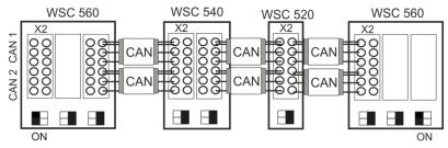
First and last bus-termination must be ON.
