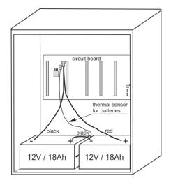
It is possible to deselect the emergency power batteries if the panel can be supplied from a 230V emergency power system such as a UPS or a 230V No-break system.
