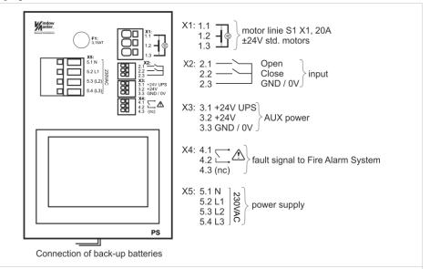
X1 For connection of ±24V standard motors (total max 20A) and espagnolette actuators type WMB 801/WMB 802/811/812/815/816/817/818.
