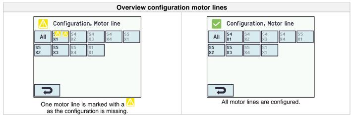
All motor outputs on the motor module as well as the single motor output S1.X1 on the WSA 5PS module are to be configured:
