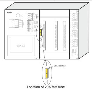
The fuse is located behind the modules. To replace the fuse, it is therefore necessary to remove the modules, see section 23.2 for replacement of modules.
