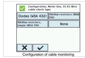
The configuration of cable monitoring must be done for each motor line.
