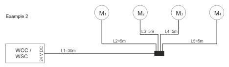
Total cable length = L1 + L2 + L3 + L4 + L5 = 30m + 5m + 5m + 5m + 5m = 50m
