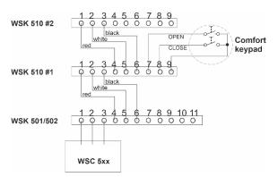
Comfort keypads can be connected to WSK 510. Smoke detectors cannot be connected to WSK 510. Please see WSK 510 instruction for configuration.
