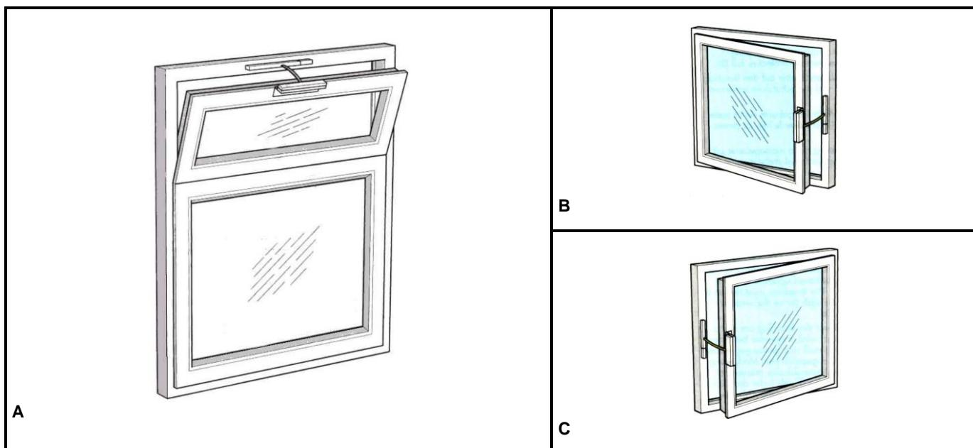
**English:** The window chain actuator can be fitted to inward opening hopper (**A**) and side hung windows hinged on the left (**B**). For windows hinged on the right (**C**) the coupling bracket must be turned as shown on page 5, ill. 17.
