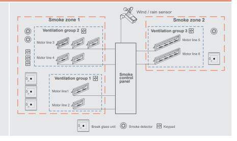
WSC 310/320 Plus smoke control panels can be used in NV Embedded<sup>®</sup> indoor climate solutions.
