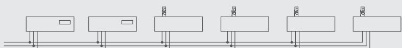
WMB 817-2 + WMB 818-2 double locking actuators with up to four quad window actuators
