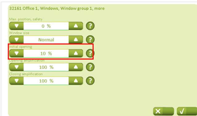
The value “Initial opening” defines the window’s opening, which must be performed at the first airing after the windows have been completely closed, e.g. to release the window’s gaskets from the frame.
