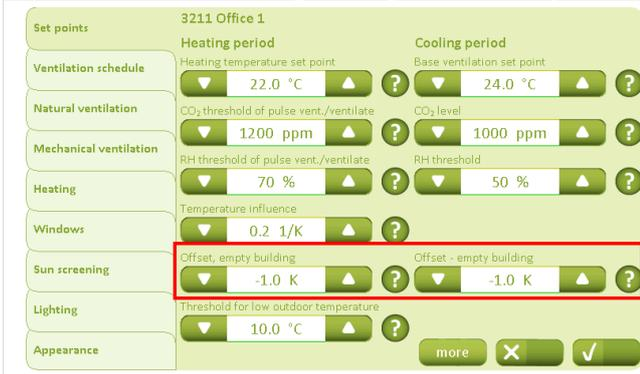
NV Comfort™ allows the lowering of the temperature set-point either to perform night cooling in summer or heat conservation in winter. The fields for temperature displacement "empty building" under the "Set-points" tab can be used for this purpose.
