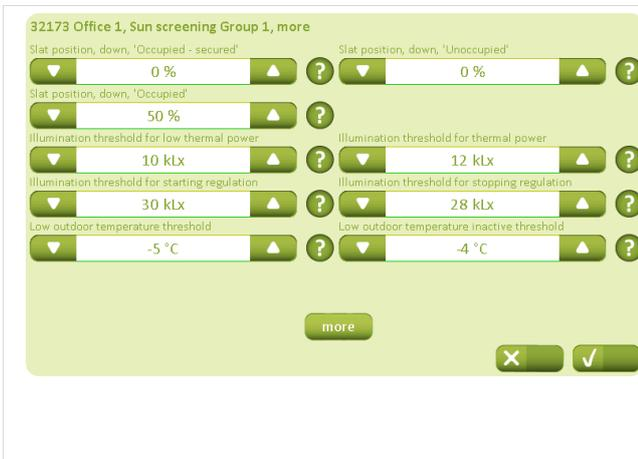
The slat position (horizontal or vertical) when the slats are deployed in the different operating modes must be defined under the tab “Sun screening” – “More”.
