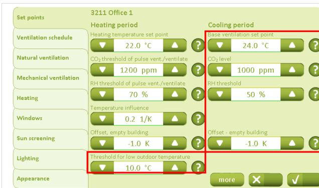
Under “Heating period”, the set-points for the winter mode can be configured. Under the “Threshold for low outdoor temperature” set-point it can be configured when to change between summer and winter mode.
