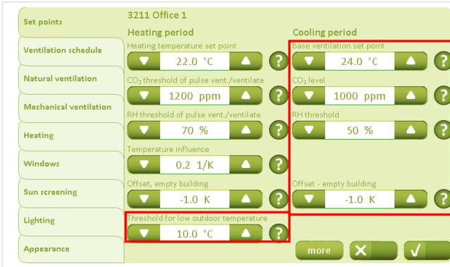
Under “Heating period”, the set-points for the winter mode can be configured. Under the “Threshold for low outdoor temperature” set-point it can be configured when to change between summer and winter mode.
