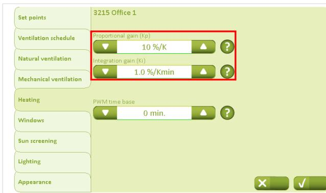
It is recommended not to set the proportional gain too high on the “Heating” tab, e.g. 50%/K, as this can result in instability/cyclic variation.
