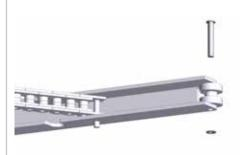
Remove the lockwasher and the pin.
