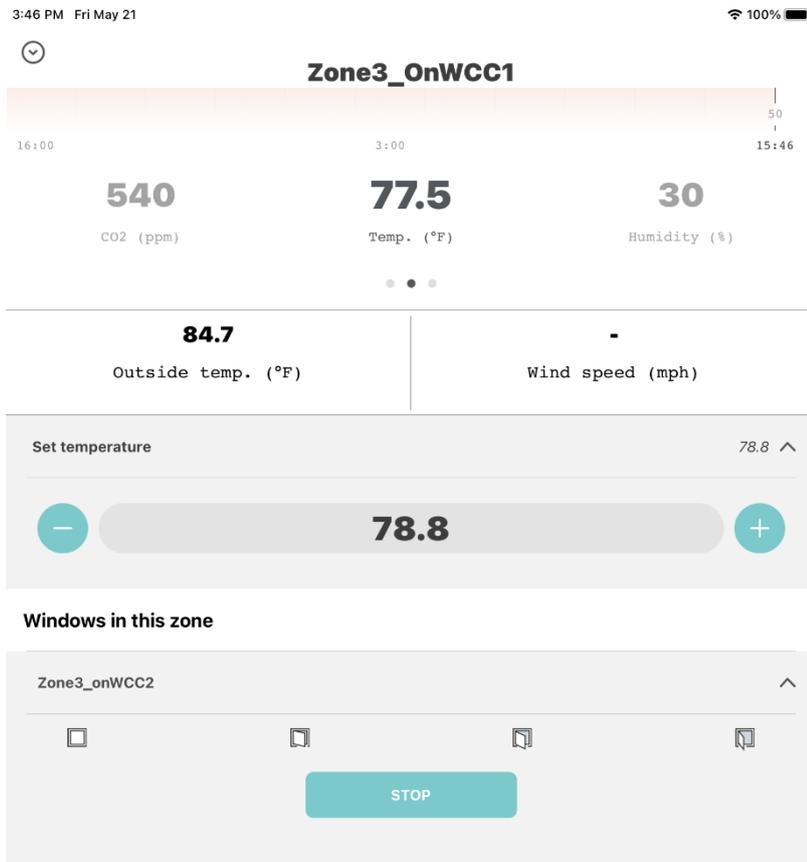
The upper part of the screen shows the last 24 hours trend of CO2, temperature and relative humidity with the current readings underneath.
