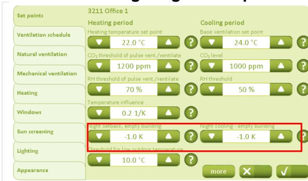
NV Comfort® allows the lowering of the temperature set-point either to perform night cooling in summer or heat conservation in winter. The fields for night setback and night cooling for “empty building” under the “Set-points” tab can be used for this purpose.
