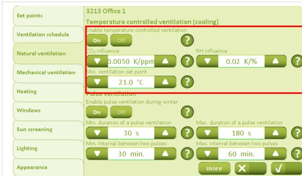
Enable whether the ventilation is to be temperature based or not. The effect of the CO<sub>2</sub> content and the relative humidity on the desired set-point to be calculated are configured under the “Natural Ventilation” tab, if the previously set limits are exceeded, the system reduces the temperature set-point in accordance with the settings.
