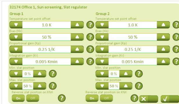
The tilting of the slats must be configured. The tilting is based on temperature measurements in the room.
