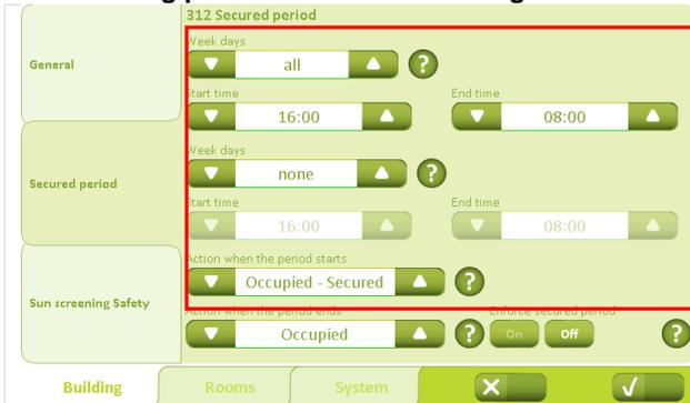
The time periods for the different operating modes must be configured here. For example, two different times can be configured: one for working days and one for weekends.
