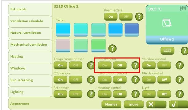
Since the ventilation is to be carried out according to the temperature, CO<sub>2</sub> and humidity, the PIR sensor, Blinds control, and light control must be set to Off.
