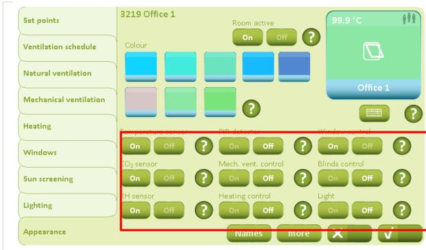
Since only one temperature-dependent ventilation is required, "CO<sub>2</sub> sensor", "RH sensor", "PIR sensor", "ventilation control" and "heating control" must be set to "Off".
