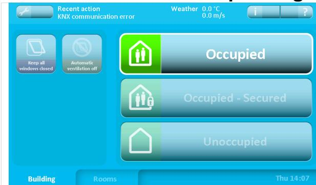
NV Comfort® has three operating modes by which the system can be configured for the current conditions. See section 2.1.1.
