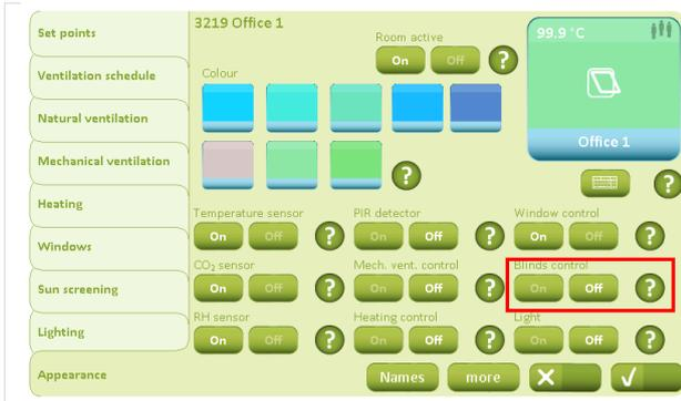
On the “Appearance” tab, “Blind control” must be set to “On” in all rooms if sun shade control is required.
