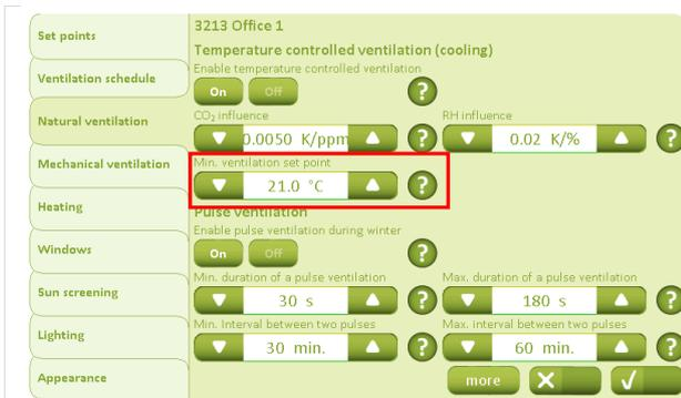
Under the “Natural Ventilation” tab, “Min. ventilation temperature set-point” defines the minimum ventilation set-point the system may use.
