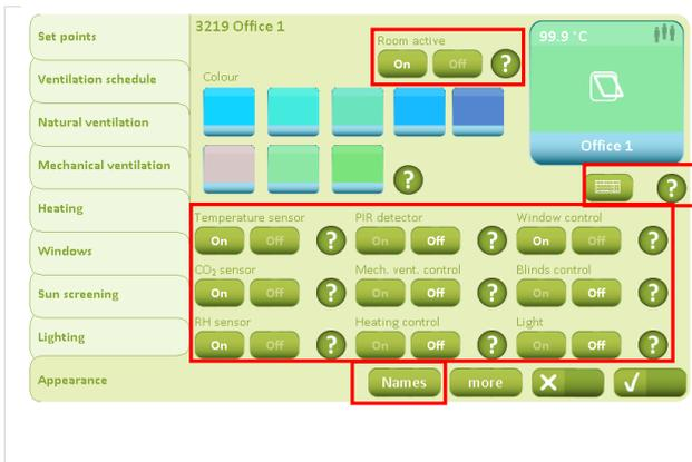
Press “On” in the room menu under the “Appearance” tab. The room is thereby activated.
