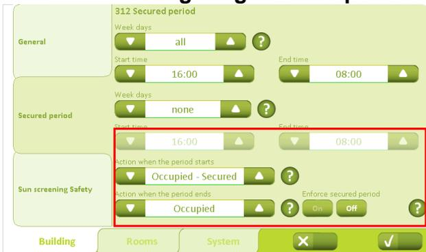
The time period for the automatic change between operating modes is configured under the “Building” – “Secured period” tab.
