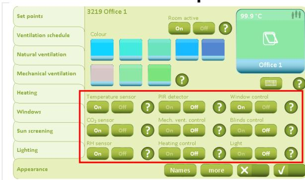
On the "Appearance" tab, the "Temperature sensor", "CO<sub>2</sub> sensor" and "RH sensor" must be set to "On" in all rooms in order to control the Natural Ventilation.
