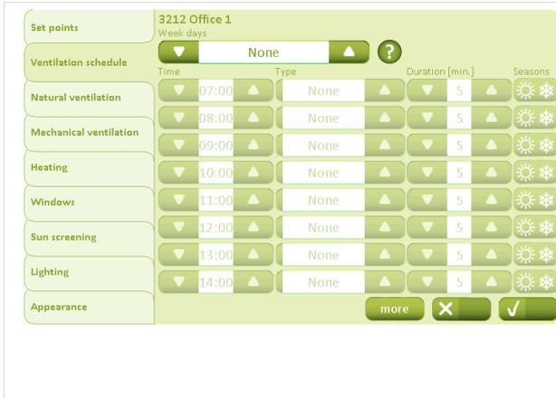
The time/length of the airing/ventilation and the time at which the ventilation should occur are configured on the “Ventilation times” tab.
