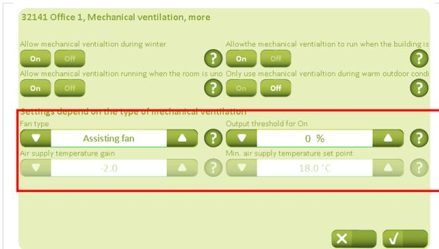
On the “Mechanical ventilation” “More” tab it is defined whether a FutureVent™ or an assisting fan is used. It is not possible to use both an assisting fan and FutureVent™!
