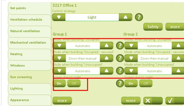
The “Sun screening” tab is used to define how the sun screen products are to be controlled in the different operating forms.
