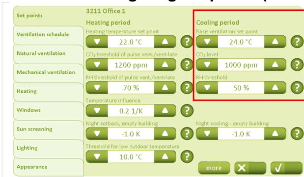
The set-points for summer operation are indicated under the “Set-points” tab and the “Cooling period” heading.
