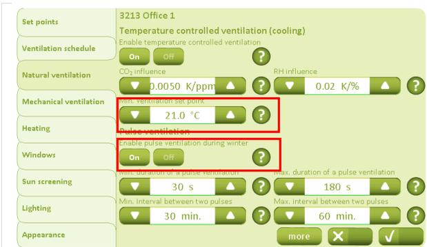
The “Minimal ventilation set-point” can be configured as required. Be aware that it must be at least 2K higher than the “Set-point for low room temperature” (screen image under “More”), as this could otherwise cause cyclical variation.
