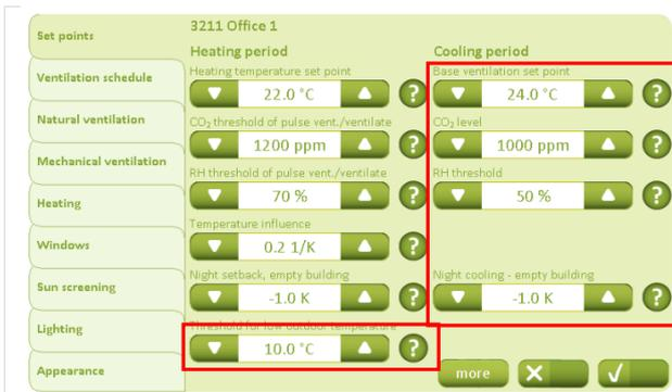
Under “Heating period”, the set-points for the winter mode can be configured. Under the “Threshold for low outdoor temperature” sep-point it can be configured when to change between summer and winter mode.
