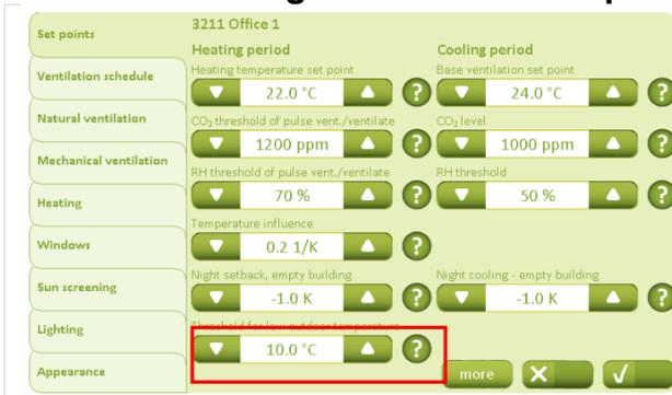
The “Set-points” tab is used to configure the “Threshold for low outdoor temperature”, which defines the temperature at which the system shifts between summer and winter operation.
