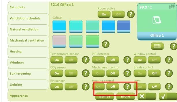
On the "Appearance" tab, "Heating control" must be set to "On" in all rooms in where heating control is required.
