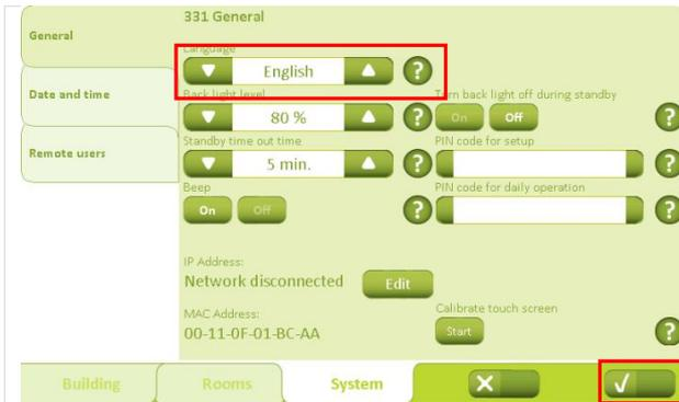
The “General” tab can be used to configure: language, background illumination, the time after which the background illumination will go into sleep mode, the beep sound when the keys are used and the PIN code for super-user and end user respectively. It is also possible to calibrate the screen image.
