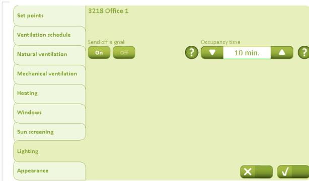
On the “Lighting control” tab, the “Send off signal” must be set to “On” in all rooms if lighting control is required.
