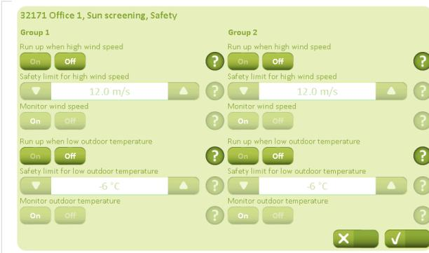
For the protection of the sun screening product, it is recommended that the sun screening product is withdrawn in the event of either high winds or low temperature.
