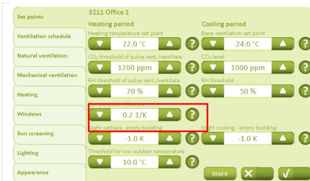
The “Temperature influence” value is used to determine whether pulse ventilation should also be used in winter when the temperature set-point, the relative humidity set-point or the CO<sub>2</sub> set-point is exceeded.
