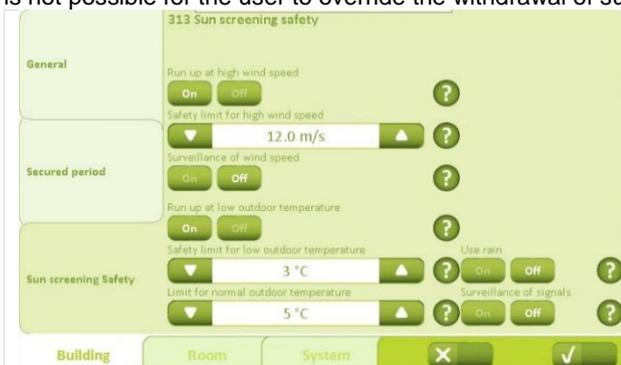
The “Sun Screening Safety” tab under “Building” is used to configure the safety set-points generally for the building.
