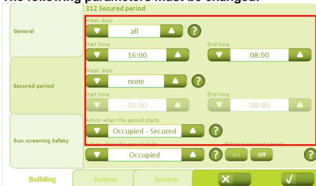
The time periods for the different operating modes must be configured here. For example, two different times can be defined: one for working days and one for weekends.
