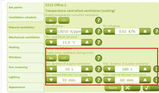
The “Natural Ventilation” tab is used to configure whether requirement-controlled pulse ventilation should be used.
