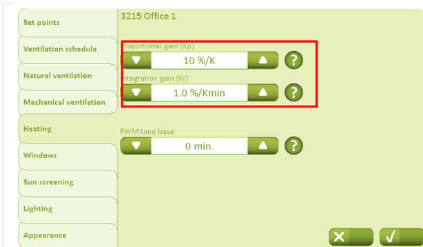
It is recommended not to set the proportional gain too high on the "Heating" tab, e.g. 50%/K, as this can result in instability/cyclic variation.
