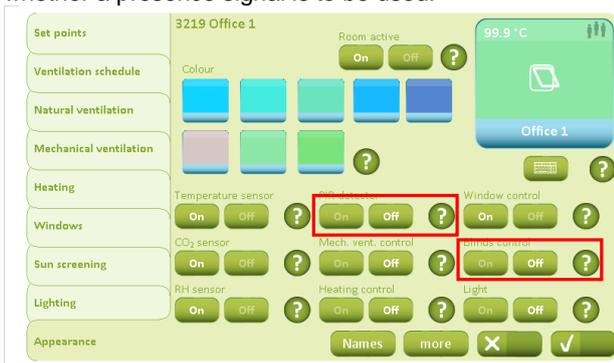
In addition to the sensors/functions that are already activated in connection with ventilation and heating control, the "Blinds control" must be set to "On".
