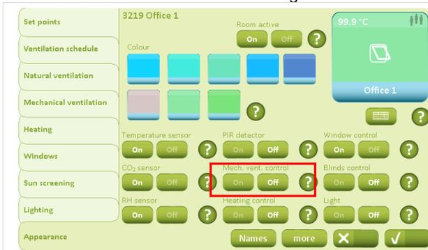
On the “Appearance” tab, “Mech. vent. control” must be set to “On” in all rooms in where control of mechanical ventilation is required.
