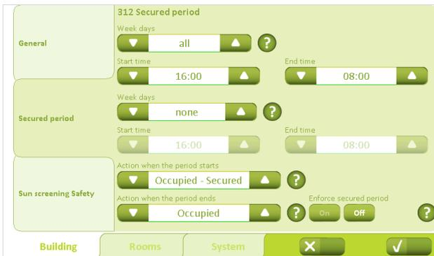
Under the “Building” – “Secured period” tab, secured periods can be defined using days and times.
