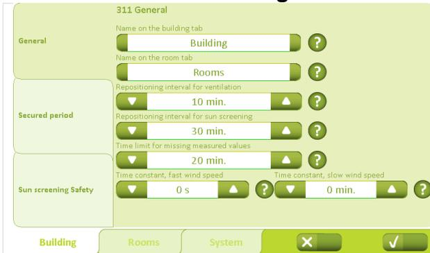
Under the “Building” – “General” tab, the building tab can be renamed and the time interval for the natural ventilation can be defined.
