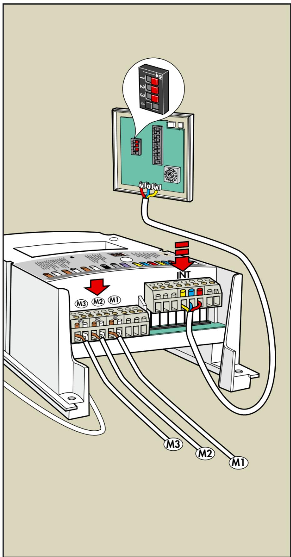
**English:** Three motors can be operated with a single function of an individual keypad; the motors will be activated in sequence. Connect keypad cable to outlet "INT" of the control unit. Switches **1, 2** and **3** of the keypad are set to the "**ON**" position.
