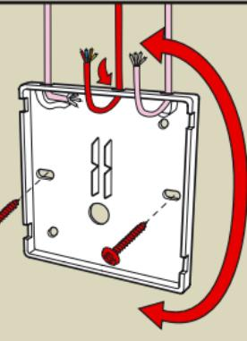
**English:** Fit keypad WLI 110 on wall. **Hidden wiring (A):** Run cable through hole in backplate. **Visible wiring (B):** Decide where to lead the cable through. Make hole in side of backplate by removing knock-out. Rotate backplate 180°, if the cable is to be led through at top of the keypad.
