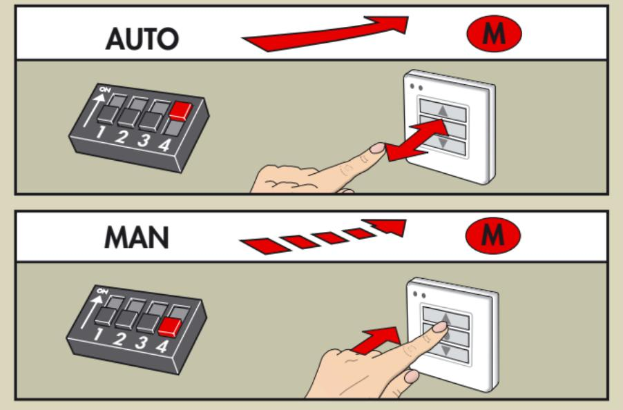
**English:** If a switch (1, 2 or 3) is set in position "**AUTO**" (automatic), the corresponding motor will travel to the end-stop after one press of the button. If a switch is set in position "**MAN**" (manual), the motor will run only as long as the button is pressed (recommended for electrically operated Venetian blind).
