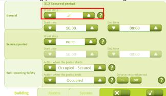
"Week days" must be changed from "all" to "none" under operating modes. In other words, there are no times where there is no ventilation if this is necessary according to the temperature.
