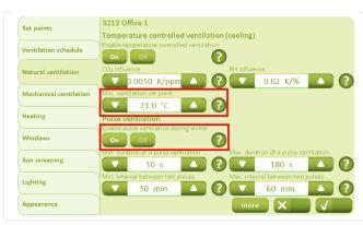
The "Minimal ventilation set-point" can be configured as required. Be aware that it must be at least 2K higher than the "Set-point for low room temperature" (screen image under "More"), as this could otherwise cause cyclical variation.
