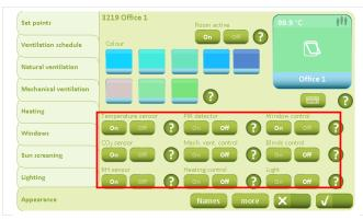
Since the ventilation is to be performed according to temperature, CO<sub>2</sub> and humidity, these sensors are set to "On", whereas the "PIR sensor", "Mech. vent. control", "Heating control", "Blinds control" and "Light control" must be set to "Off".
