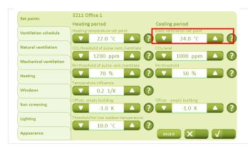
In the "Cooling period", the "Basic ventilation set-point" can be defined for the each room as required.
