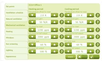
Parameters for temperature, CO<sub>2</sub> and RH effect on the mechanical ventilation can be adjusted as required.
