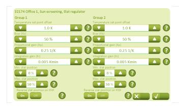
The tilting of the slats must be configured. The tilting is based on temperature measurements in the room.
