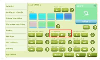
Since the ventilation is to be carried out according to the temperature, CO<sub>2</sub> and humidity, the PIR sensor, Blinds control, and light control must be set to Off.
