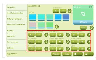
Since only one temperature-dependent ventilation is required, " $CO_2$  sensor", "RH sensor", "PIR sensor", "ventilation control" and "heating control" must be set to "Off".
