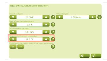
The "Threshold for low room temperature" must be at least 2K lower than the "Minimal ventilation set-point" that has just been set.
