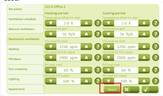
The mechanical ventilation set-points for the heating and cooling period must be defined. The set-point for "Temperature offset for start" is based on the ventilation temperature set-point, which is defined under "Set-points".
