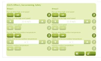
For the protection of the sun screening product, it is recommended that the sun screening product is withdrawn in the event of either high winds or low temperature.
