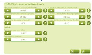
Temperature and illumination set-points must be defined based on when they contribute positively or negatively to the building's room temperature.
