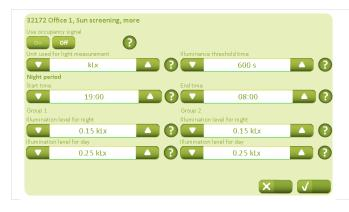
If a PIR sensor is used, "Use occupancy signal" must be set to "On".
