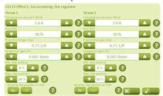
The position of the slats in the different operating modes must be configured.
