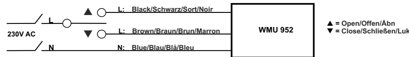
**Important!** According to national regulation, EN 60204-1 and the directive of machinery, the yellow-green cable must not be used for anything else than earth (PE).
