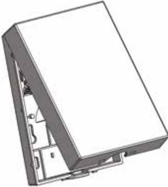
Open the box at the bottom and remove the front cover! Unplug the ribbon cable
