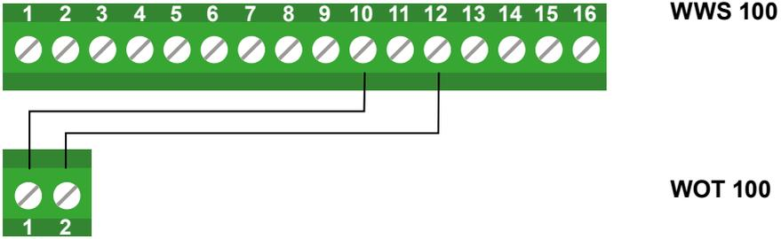
The outdoor temperature sensor WOT 100 is connected to #10 and #12 Sensor input 3 and GND respectively on WWS 100.
