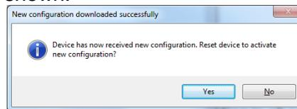
If “Yes” is pressed the WBA device is reset. It will disappear from the device list until it is discovered again.
