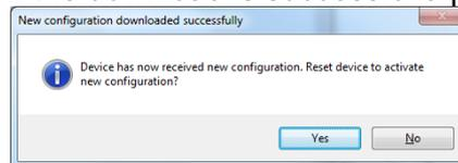
If "Yes" is pressed the WBA controller is reset. It will disappear from the device list until it is discovered again.
