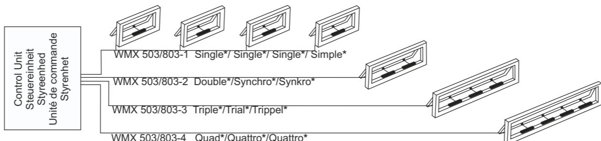
\* Up to two espagnolette actuators type WMB 81x-n can be installed on a window (max. one single or two double WMBs on each motor line) - see product sheet for valid actuator combinations.
