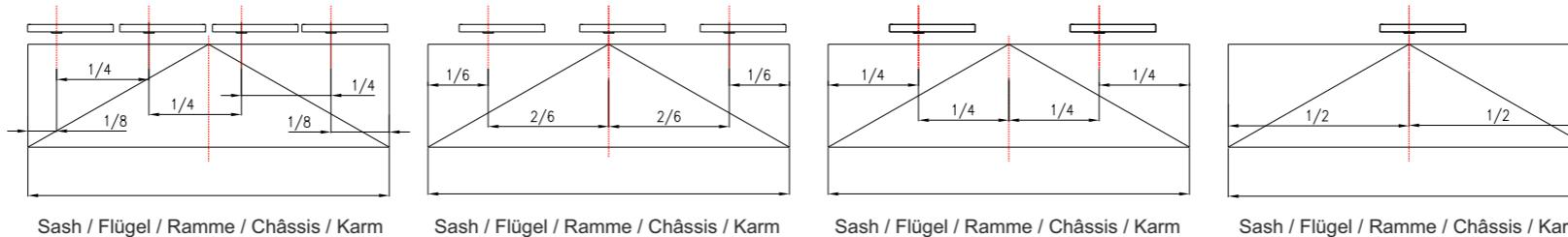
Distribution of window actuator / actuators in the window sash
